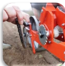
Density adjustment by sprockets (No tools, with simple adjustment table)
