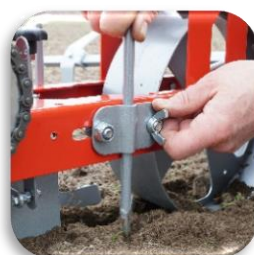
Covering skimmers with Adjustable blade-height, orientation... & removable quickly and without tools
