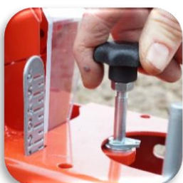
Depth adjustment by depth-screw + depth indicator
