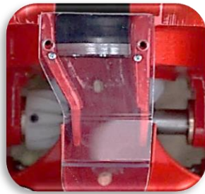
Chute with high-visibility to monitor correct distribution of seeds
