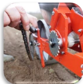
Density adjustment by sprockets (no tools, with simple adjustment table)
