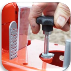
Depth adjustment by depth-screw + depth indicator
