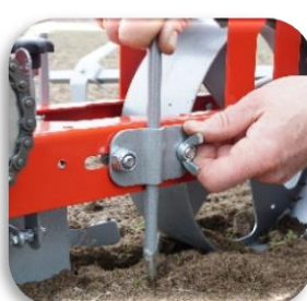
Covering skimmers with adjustable blade-height, orientation... & removable quickly and without tools Model Presented: SJ Expert
